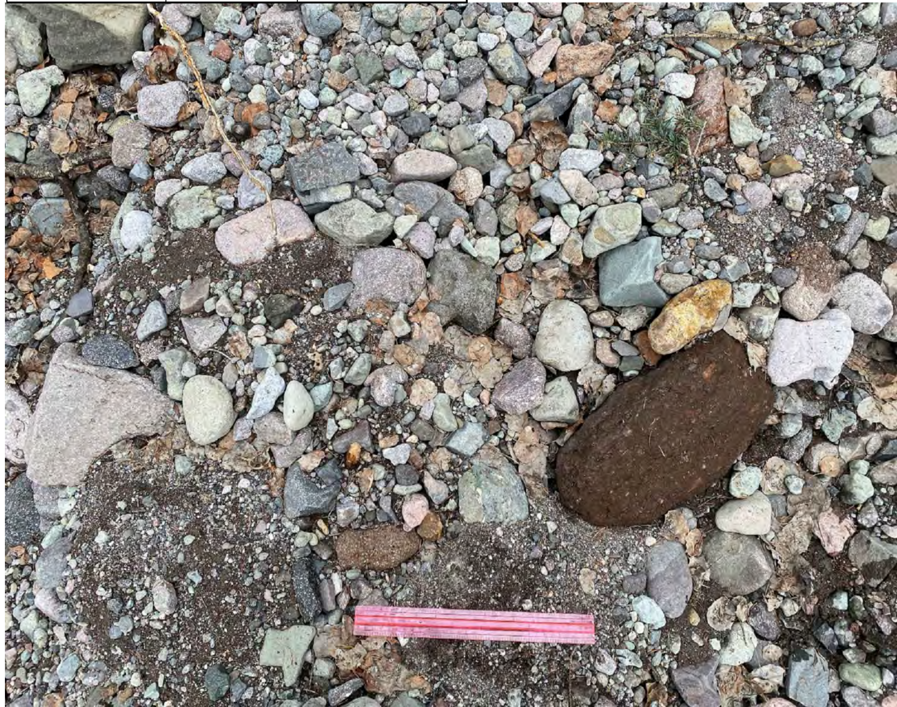
FIGURE 2: EXAMPLE IMAGE OF NATIVE ALLUVIUM MIX
